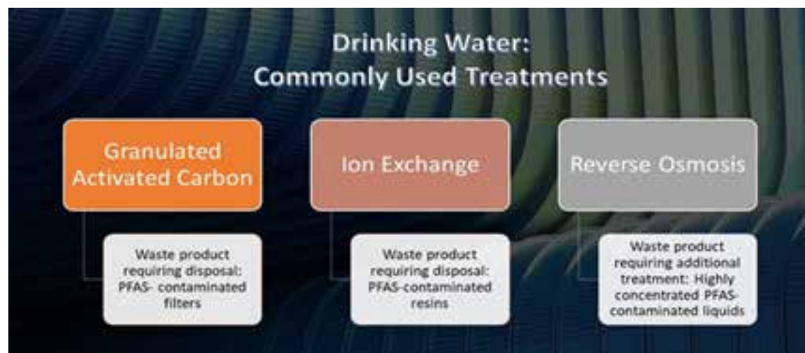
Figure 4: Commonly used PFAS treatments. Primary considerations for choosing a treatment system include, but are not limited to: cost, reliability, flexibility, and waste generation/management.
