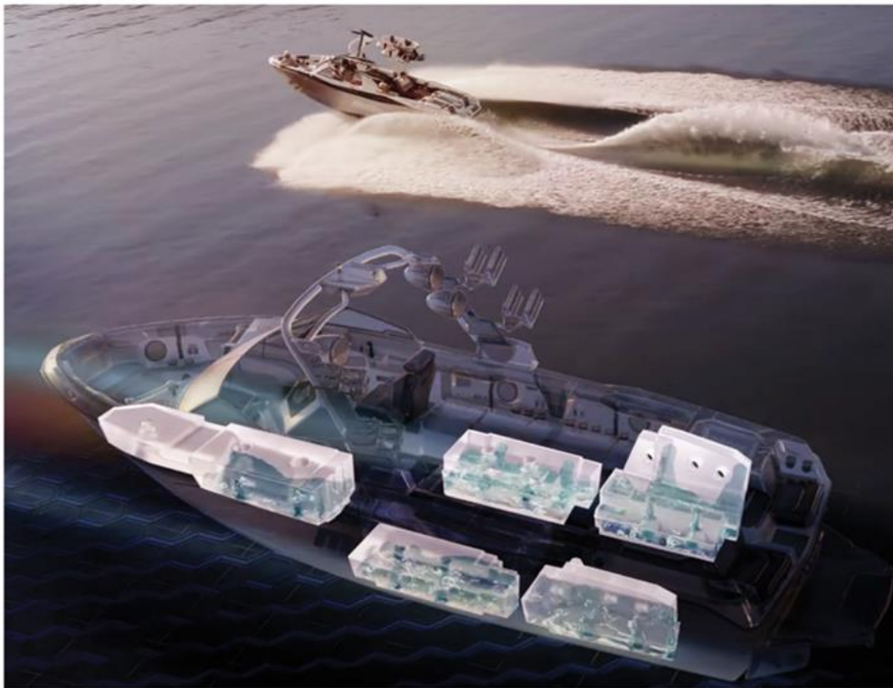
Figure 1. Internal ballast system of 2023 Malibu 26 LSV model wake boat. Image from 2023 Malibu Boats product guide. The image highlights the large volume of water held within the internal ballast system with minimal access to decontaminate.
