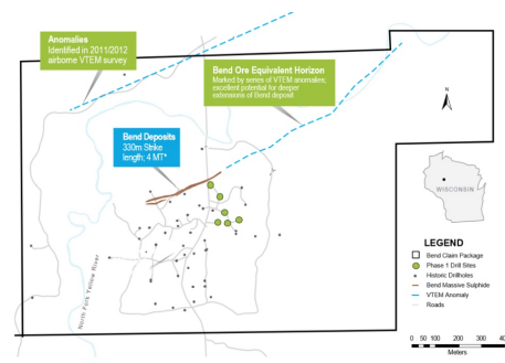
Figure 1 – Plan view of the Bend Project showing Phase 1 drill hole locations (green circles) targeting extensions along the eastern margin of the deposit.
